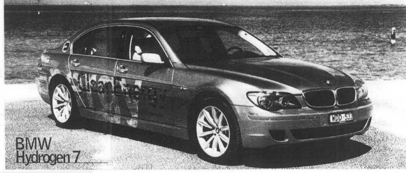
safety vents. Store the car for six weeks, and about half the hydrogen in the tank will eventually escape through the vents, even though the tank's insulation is so good that it will keep ice frozen for 13 years.
